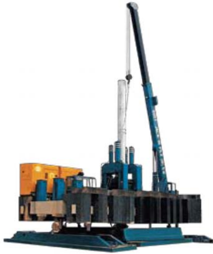
600 tons hydraulic Jack-in machines with crane.
