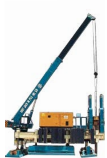
380 tons hydraulic Jack-in machines with crane.
