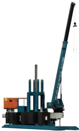
250 tons hydraulic Jack-in machines with crane.
